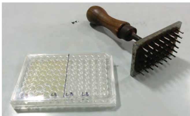
Fig. 1: Creating a master plate using a modified metal stamp and a 96 well plate
