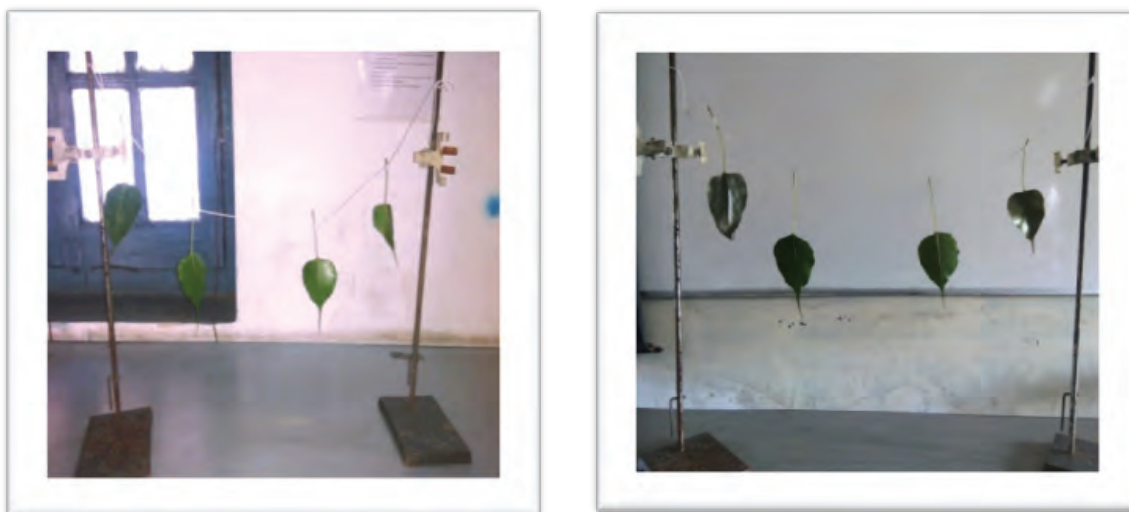
Fig. 2: Loss of water from two surfaces of leaf by four leaf method.
